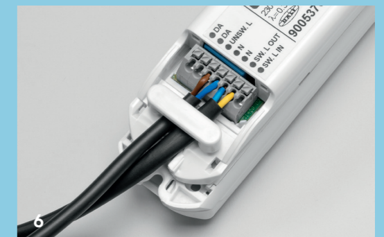
6 Connect the mains cable to the emergency LED driver (neutral conductor and unswitched line) and fix the cables with the strain relief.
